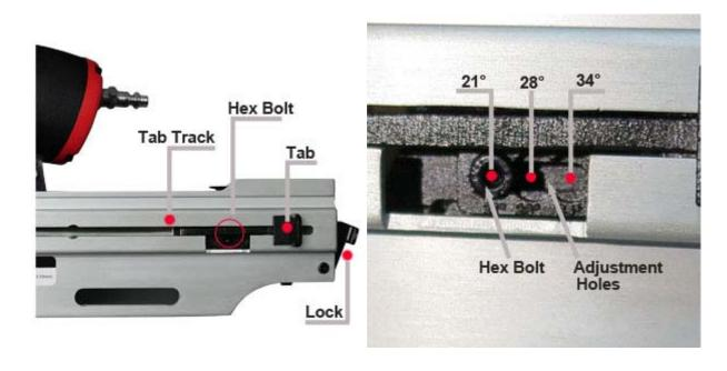
Pull back and engage the Tab, exposing three adjustment holes. Loosen the hex bolt and slide it into the appropriate hole (21°, 28°, 34°). Retighten the hex bolt, making sure it fits into the appropriate hole properly. When done, carefully release Lock while guiding the Tab towards the front with your hand.
